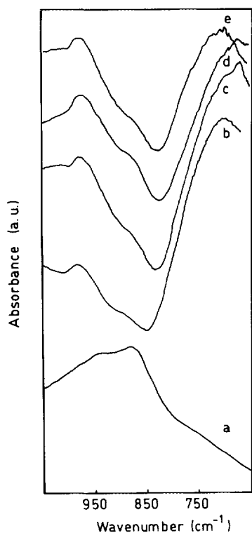
FIG. 7. FTIR spectra of the supported phases (KBr pressed disks, support spectrum subtracted) of V 2 O 5 (1.4)/TiO 2 (a), WO 3 (9)/TiO 2 (b), V 2 O 5 -WO 3 (9)/TiO 2 samples with V 2 O 5 = 0.3% w/w (c), 1.0% w/w (d), and 1.4% w/w (e).
